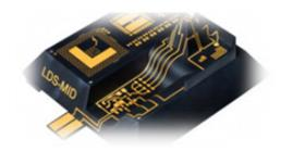
LDS antenna technology is mainly used in the field of mobile communication to realize the functions of smart phone antenna and mobile payment.
